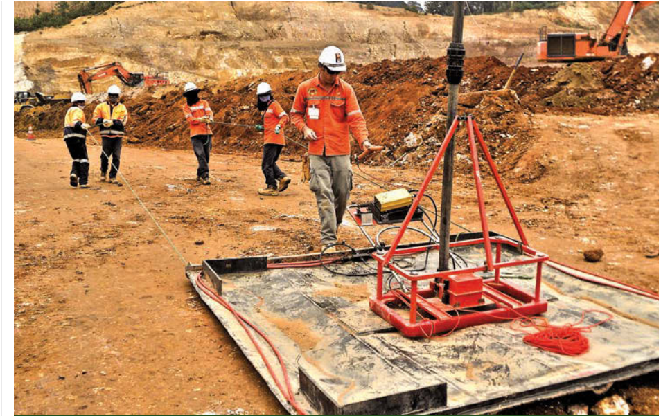
Laneville directs his team in dragging his mine-detecting device (Modified EM61 with 2-turn transmitter) near mineral exploration sites around Sepon, Laos, home of the country's largest gold and copper mine.
